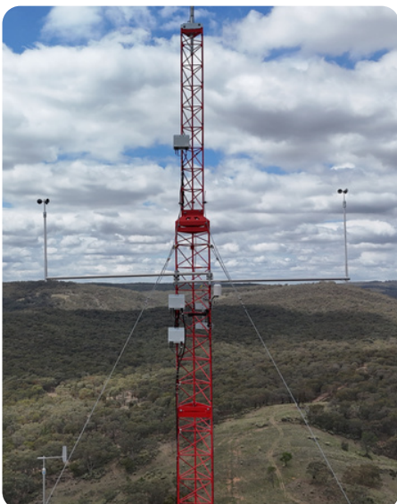
Figure 2: Example of sensors installed on a meteorological mast
