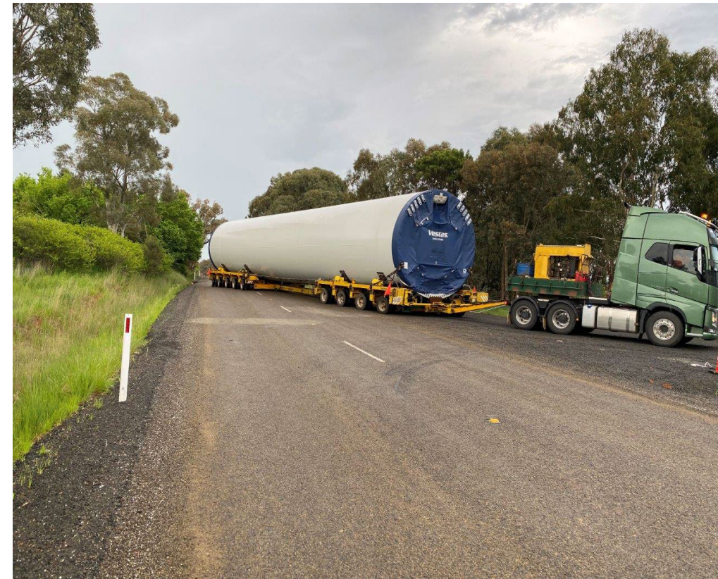
First Tower Section Delivery
