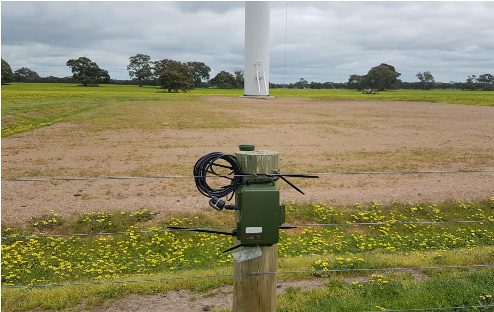
Figure 2 SM4 detector mounted on a fence near Turbine 13
