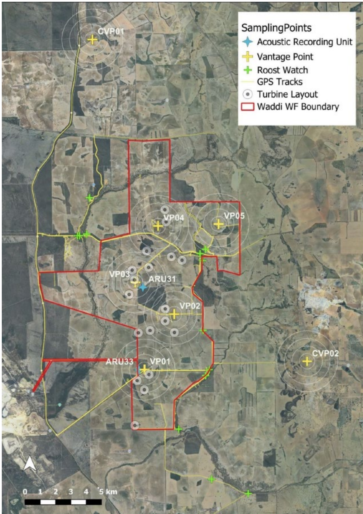
Figure 3: Sampling points and recording unit locations for Waddi Wind Farm, with GPS tracks for the surveyors recorded throughout campaigns
