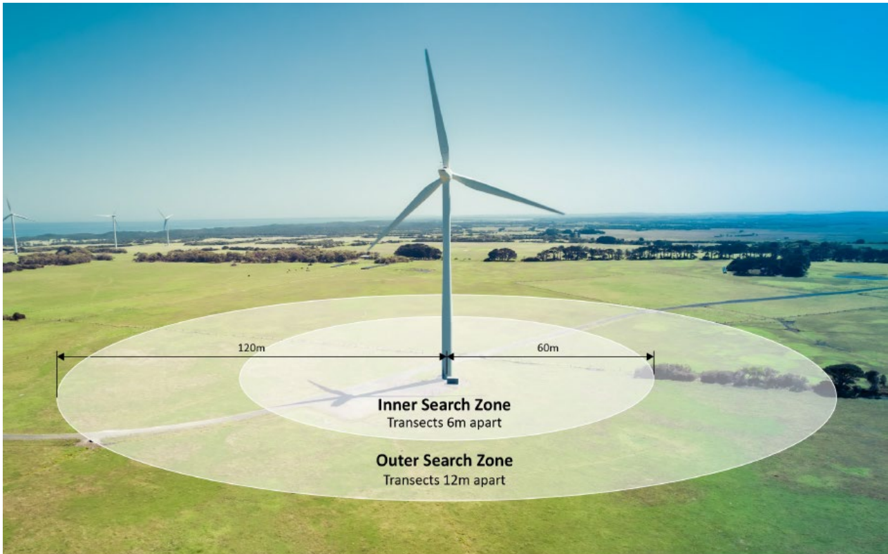
Figure 7: Inner and outer carcass search zones underneath turbines
