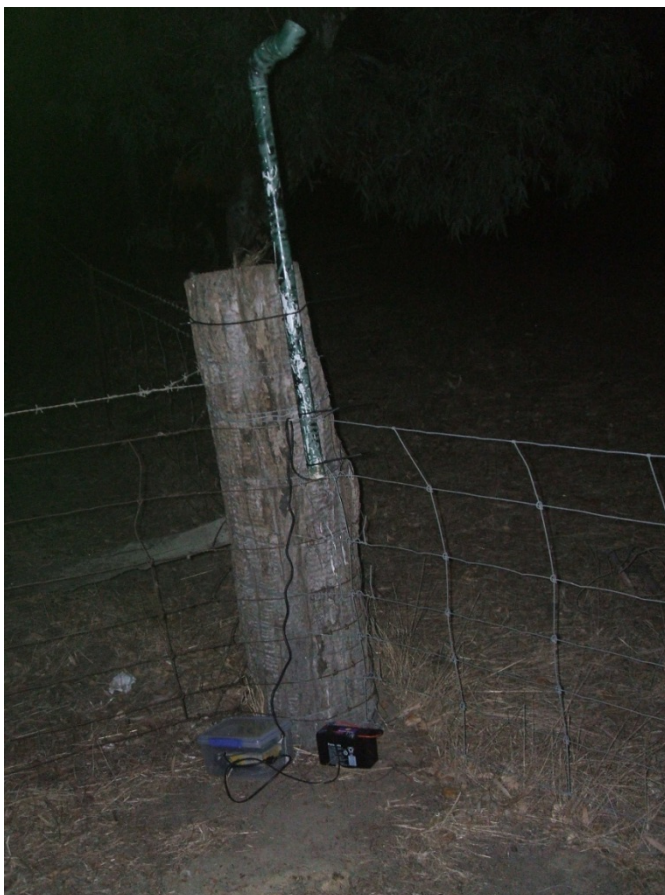
Plate 2: Bat Detector and Microphone Protector located at Sampling Point W1
